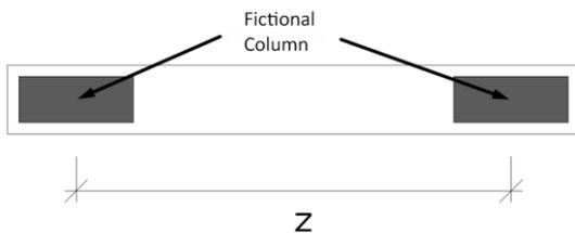
Figure 7.3 - Schematic representation of a shear wall, including the end elements and the bending arm, z.
