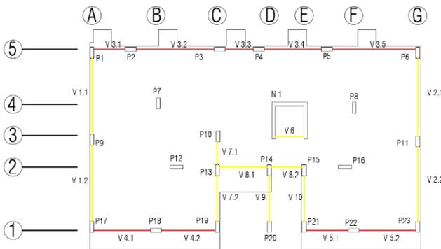
Figure 4.1 - Location of beams and columns in plan.
