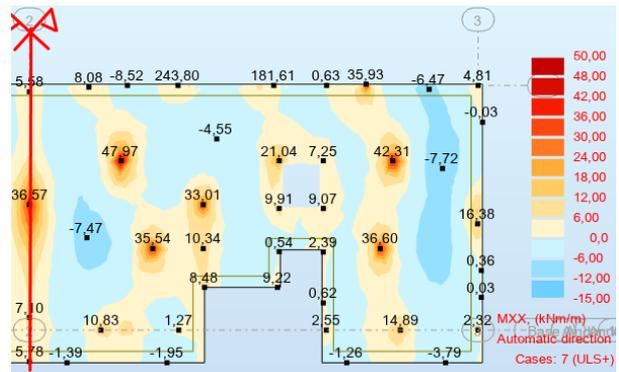
Figure 7.1 - Map of bending moments, in the x direction, fundamental combination.
