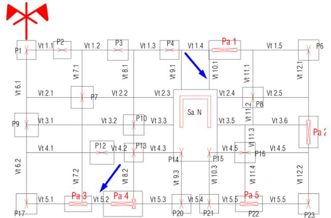
Figure 7.4 - Schematic indication of the location of maximum bending moments in the tie-beams.
