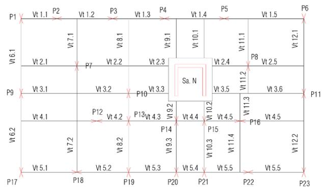
Figure 4.2 – Tie-beams disposition, Vt, in the case of the seismic joint model.
