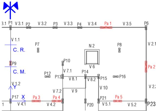
Figure 6.1 – Representation, in plan, of the location of the structural elements.
