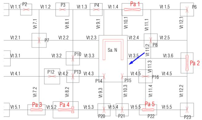
Figure 6.2 - Location of the footing that incorporates the spread footing of the two columns and the one of the nucleus.
