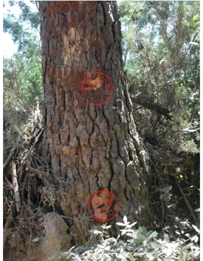
Fig. 4. Configuration of the electrical tree resistance measurements: a- R_{tree} b- R_{x1-x2}
