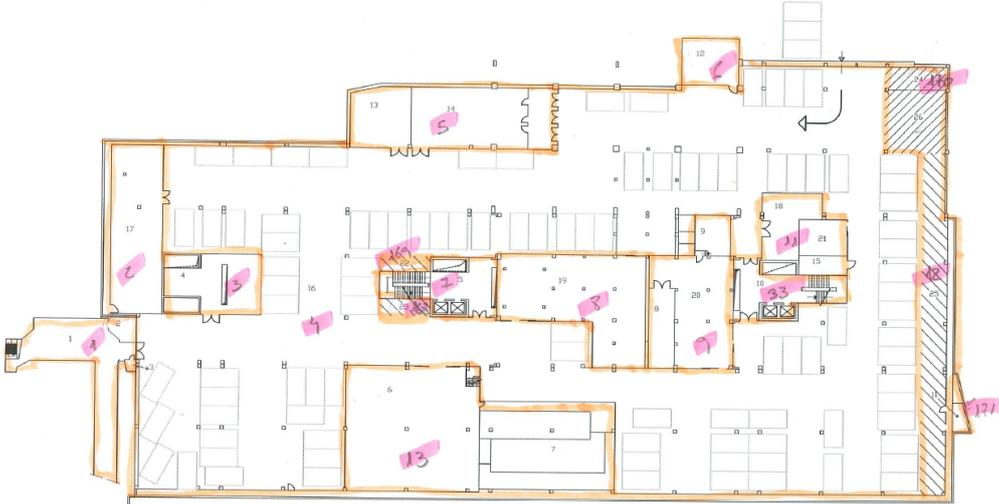
Figure A.1: Thermal zones of the 03 floor.
