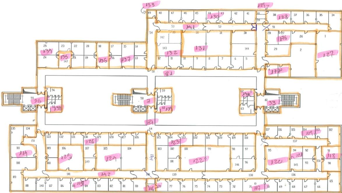
Figure A.6: Thermal zones of the 2<sup>nd</sup> floor.
