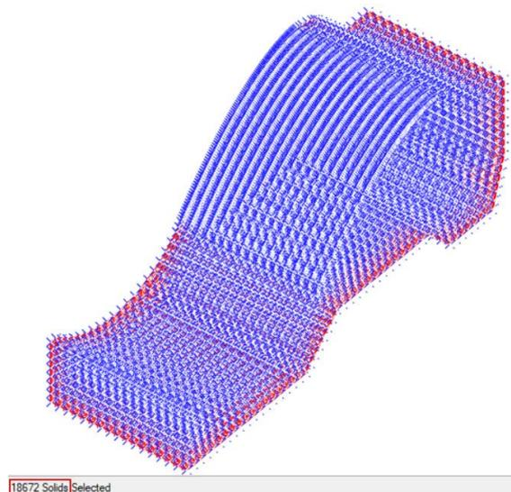
**Figure 19:** Converted mesh imported to SAP2000 (18672 solid elements selected)
