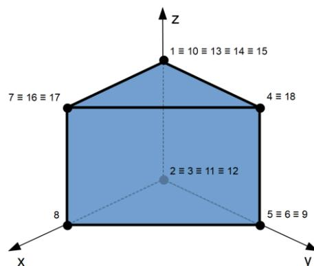
**Figure 7:** Triangular prism, 6x3 Polygon Mesh element
