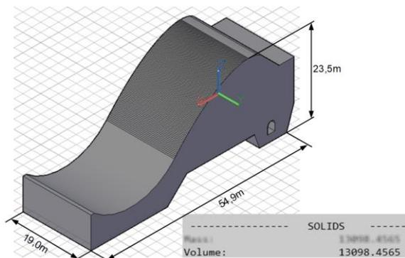
**Figure 16:** WES spillway solid model and its volume, approximately equal to  $13098,5\text{m}^3$  (AutoCAD)
