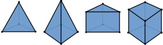
**Figure 4:** Types of linear elements generally used in 3D mesh generation
