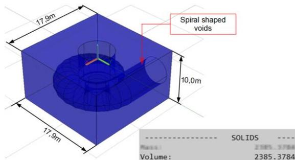
**Figure 10:** Spiral case solid model and its volume, approximately equal to 2385,4m<sup>3</sup> (*AutoCAD*)
