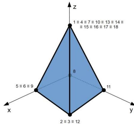
**Figure 6:** 5-node pyramid, 6x3 Polygon Mesh element
