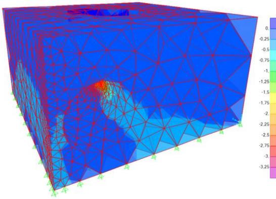
**Figure 14:** Vertical stresses for FE model, in MPa (SAP2000)
