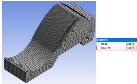
**Figure 17:** Mesh composed of 18672 triangular prismatic and hexahedral elements (Ansys Student)
