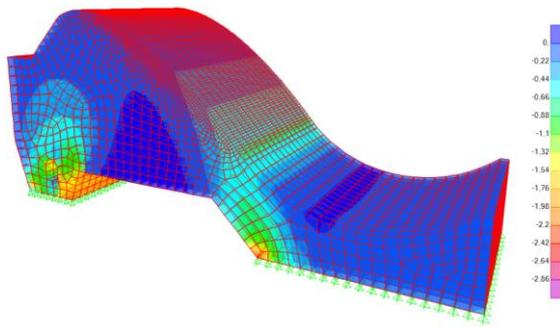
**Figure 20:** Vertical stresses for FE model, in MPa (SAP2000)
