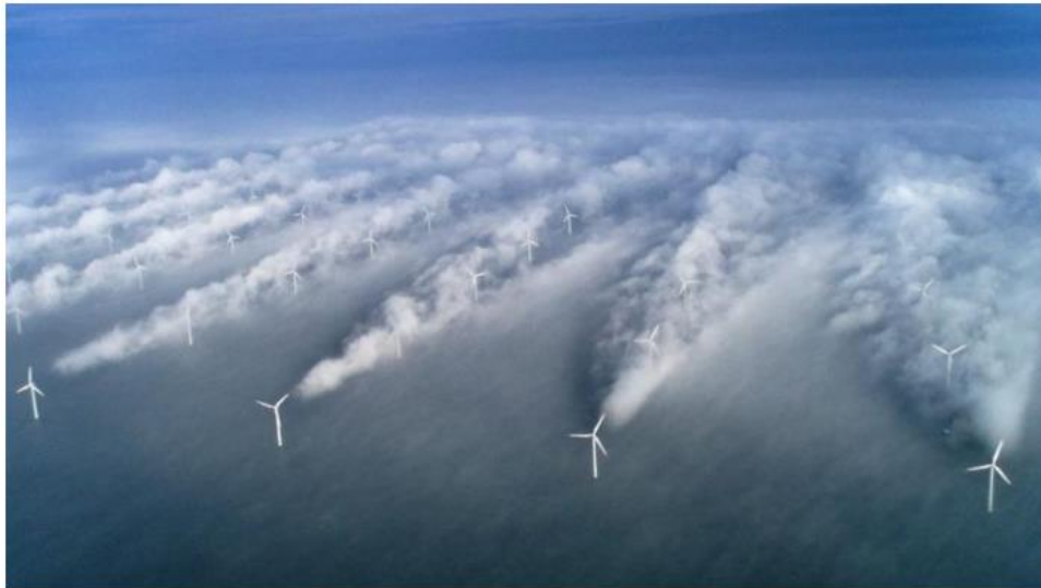
Figure 3-5: Wakes at Horns Rev wind farm made visible by weather conditions [30]
