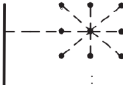
Figure 3-14: Star cable connection design [41]
