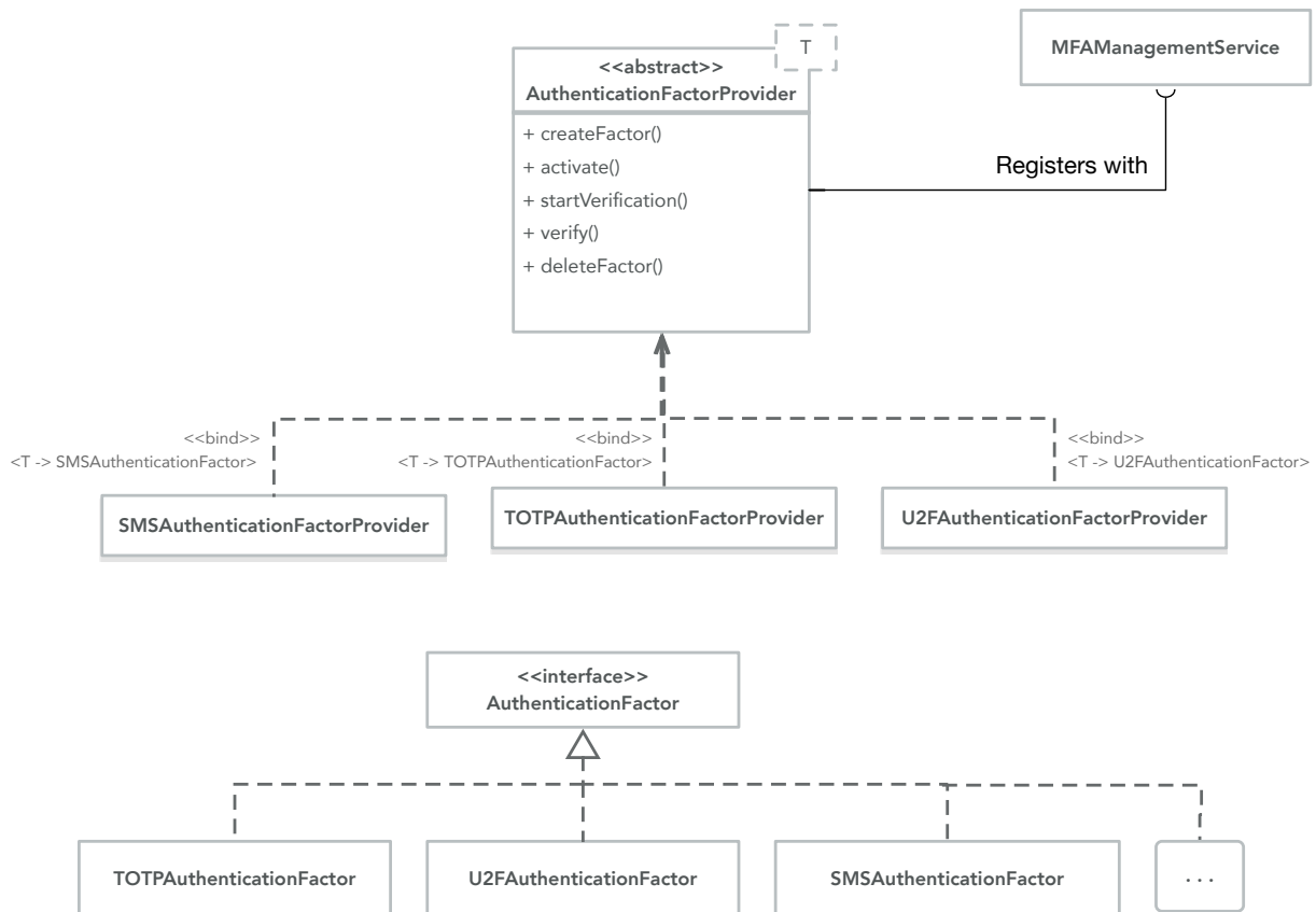
Figure 3.6: A UML representation of the classes that implement the 2FA subsystem.
