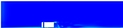
Figure 8: Contours of the f_k ratio of the dynamic simulation results at \beta = 8.8^\circ (clockwise rotation), on the plane y = 0 for the unactuated case. Blue represents f_k = 0 .
