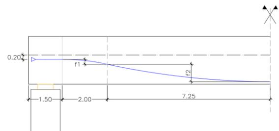
Figure 5 - Pre-stress layouts for beams A and K
