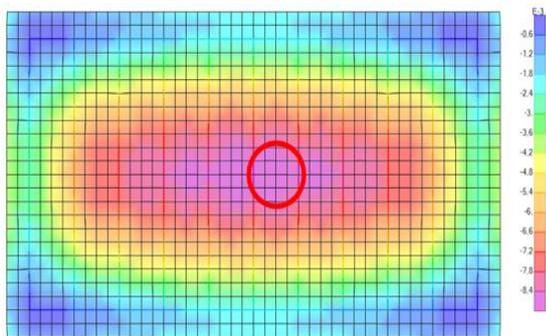
Figure 2 – Elastic deformation on the roof slab
