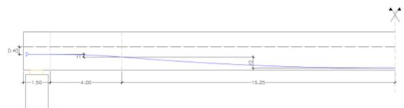
Figure 4 - Figure 5 – Pre-stress layouts for the bottom level of anchorage in beams 1 and 2
