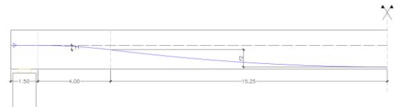
Figure 3 – Pre-stress layouts for the upper level of anchorage in beams 1 and 2
