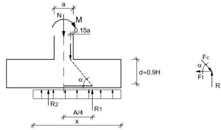
Figure 4 – Model of strut-and-tie considered in the foundations
