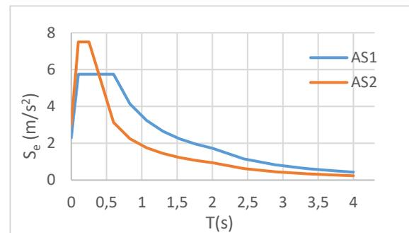
Figure 1 - Elastic response spectrum for zone 3
