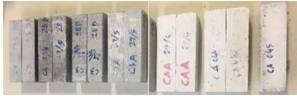
Figure 2.4-I- Prismatic specimens of a) OPC and b) amorphous binder mortar mixtures
