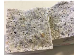
Figure 2.4-II- Failure zone of the amorphous binder specimen.
