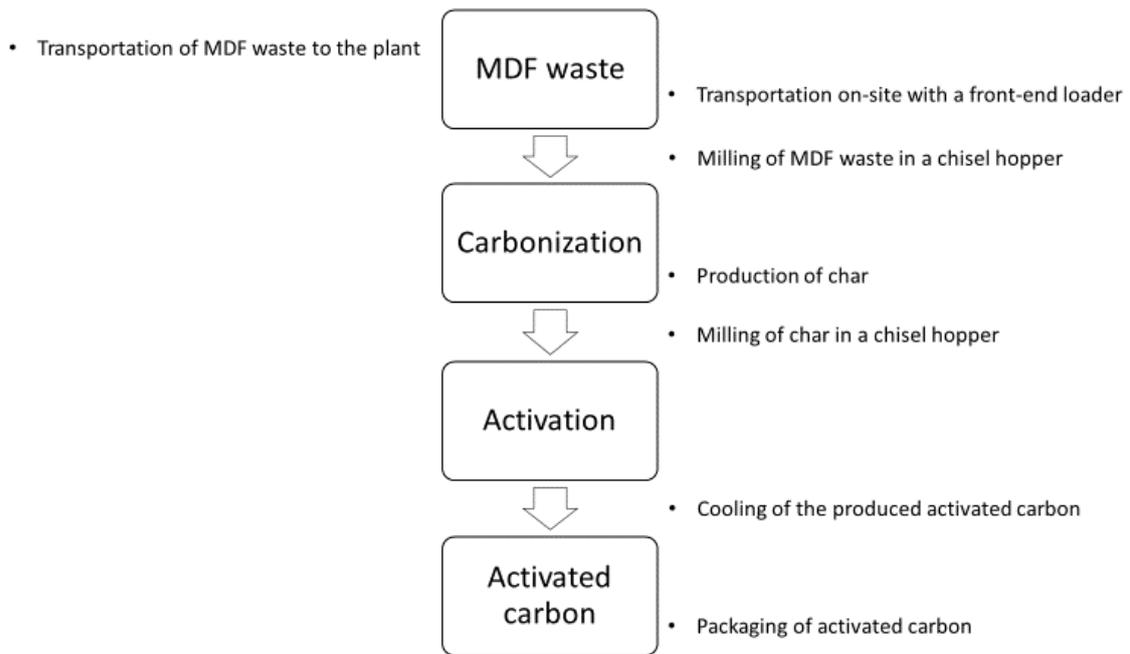
*Figure 3.1 Simplified process flow diagram of producing activated carbon from MDF waste*
