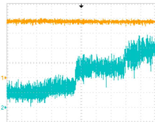
Fig. 13 - Transient response of DC grid voltage and current when the two laptops are connected to the DC grid CH1 (Orange): DC grid voltage (5V/div) CH2 (Blue): Inductor's current waveform (0.5A/div) t (50ms/div)
