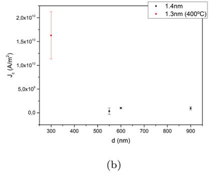
Figure 11: Critical current density  $J_c$  calculated from R(I) measurements, as a function of buffer/spacer structure (top) and of free layer thickness (bottom).
