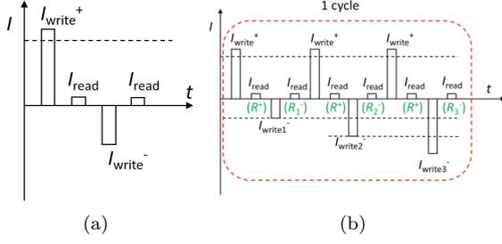
Figure 4: Measurement method for resistance states (pulse width=500ms). Left: measurement method for resistance state at given current; Right: cycle for measurement of all resistance states for a given sample.
