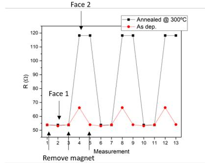
Figure 2: Example of resistance measurement with permanent magnet, showing where face 1 and face 2 are put close to the sample, as well as where the magnet is removed.
