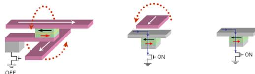
Figure 1: Comparison between MRAM architectures. Left: Conventional MRAM; Center: Thermally assisted MRAM; Right: Spin-transfer torque MRAM.
