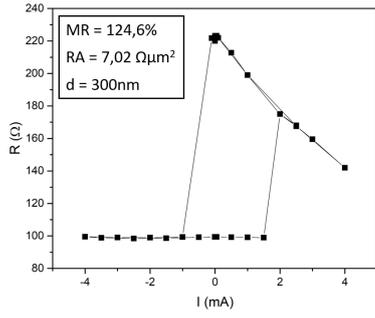
Figure 8: R(I) curve measured for sample w/ FL 1.3nm, W/W, annealed post deposition at 400°C.
