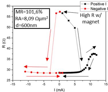
Figure 6: Example R(I) curve of sample w/ FL 1.3nm, W/Ta, annealed at  $320^\circ C$ .
