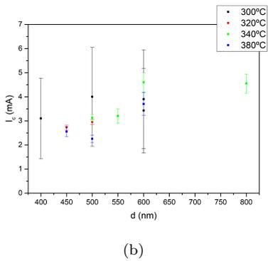
Figure 10: Calculated  $I_c$  values from R(I) measurements of sample w/ FL 1.3nm, W/Ta (top) and Ta/W (bottom), for the tested annealing temperatures.
