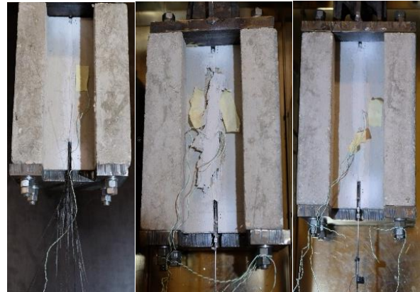
Figure 9 - Failure modes from the epoxy adhesive series without strain gauges along the connection; (a) CFRP strip rupture; (b) rupture in the adhesive-CFRP interface, with slip of the CFRP strip and posterior rupture in the adhesive-concrete interface; (c) rupture in the adhesive-CFRP interface, with slip of the CFRP strip.
