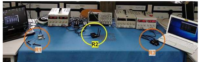
Figure 6 – Configuration of the experimental tests performed on pDDL2450 radios.
