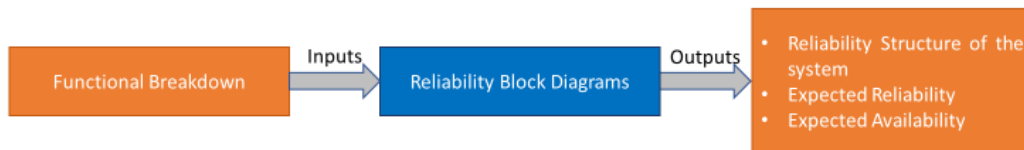
Figure 2-7: Information flow: Inputs and Outputs expected from a Reliability Block Diagram.
