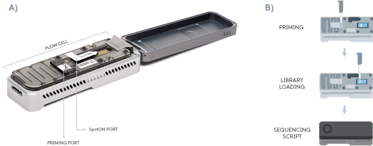
Fig. 17 - The MinION MK1B structure (A) and setup scheme (B). Adapted from: Oxford Nanopore Technologies
