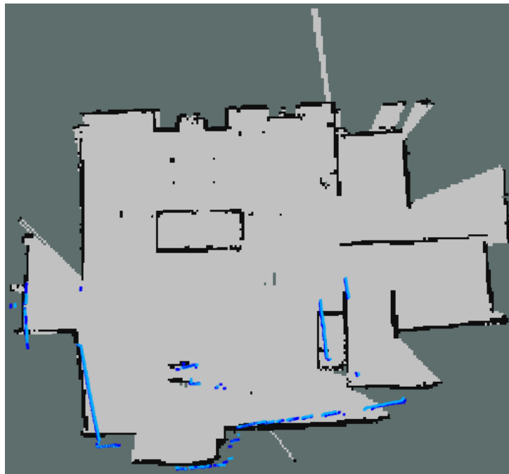
Figure 3.3: Conversion of laser scan to point cloud. Example of when the robot starts to get lost
