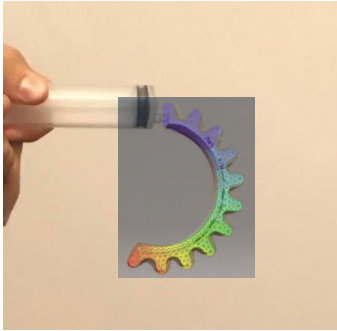
Figure 3.5 – Comparison between the real model and the ABAQUS® model
