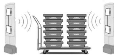
Figure 5 – Warehouse module: RFID gateway.
