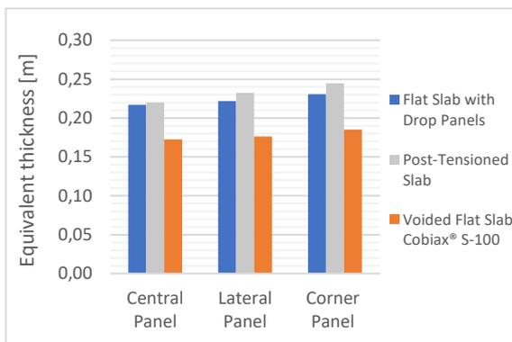
Figure 14 – Equivalent thickness for parking loads
