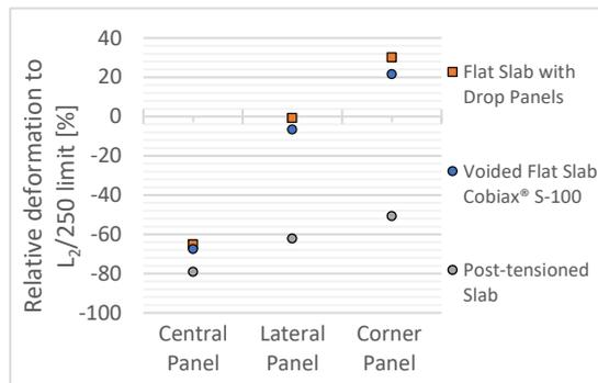
Figure 17 – long term deformation in parking structures
