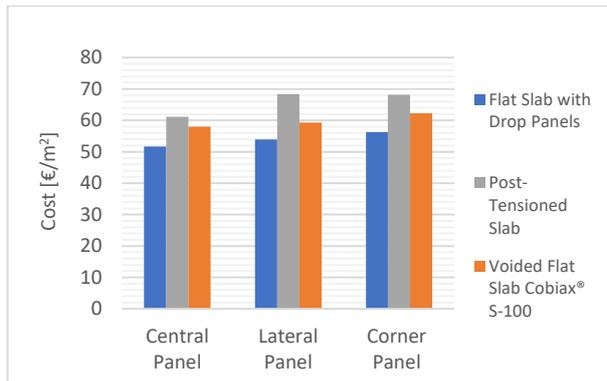
Figure 19 - Slab cost/m<sup>2</sup> for parking buildings
