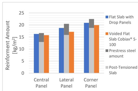
Figure 15 – Reinforcement amount for parking loads
