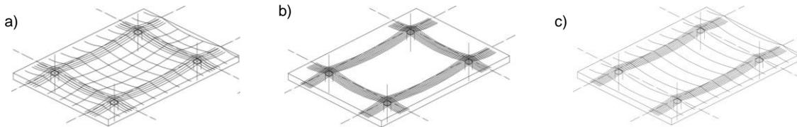
Figure 3 -Possible tendon arrangements: a); mixed distribution b) concentrated in both directions; c) – concentrated in one direction and distributed in the other.
