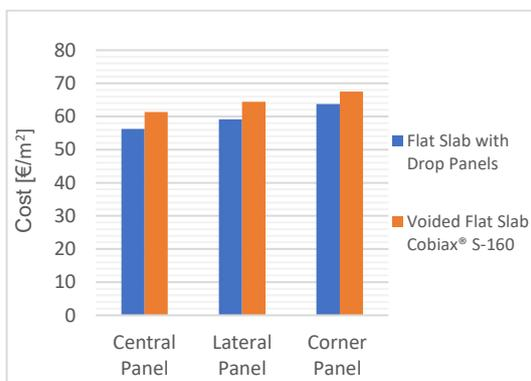
Figure 18 - Slab cost/m<sup>2</sup> for apartment buildings
