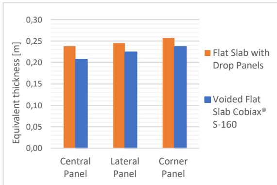
Figure 8 – Equivalent thickness in apartment buildings
