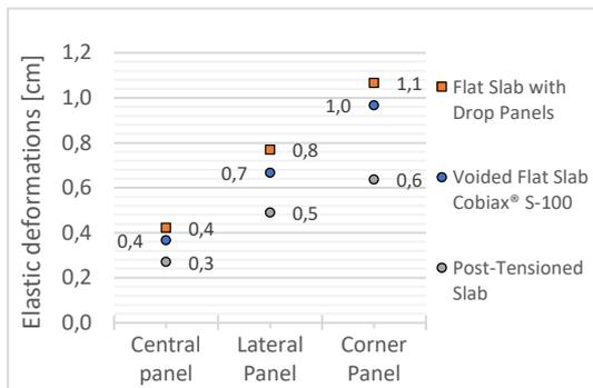
Figure 16 – Elastic deformations in parking structures
