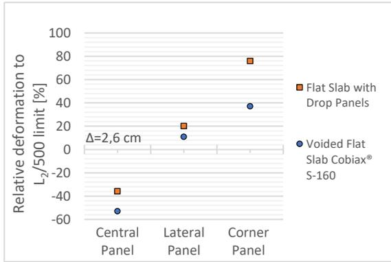
Figure 12 – Relative deformation to L/500 limit
