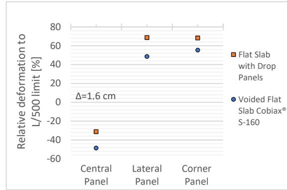
Figure 13– Relative deformation to L/500 limit
