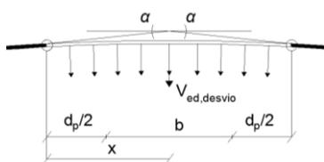
Figure 4 – decompression force in punching resistance
