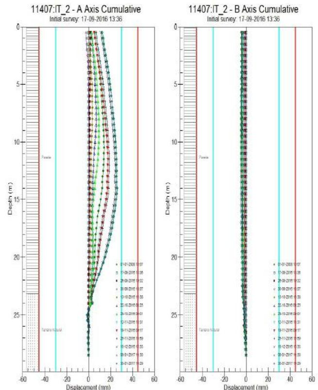
Figure 6 – Horizontal displacements measured in the inclinometer installed in the studied section: max = 25 mm (Teixeira Duarte, 2017)
