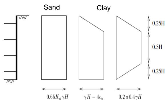
Figure 1 – Earth pressures diagram acting in flexible retaining wall
