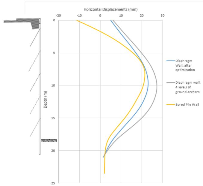
Figure 11 – Horizontal displacement in depth for different solutions presented in this paper
