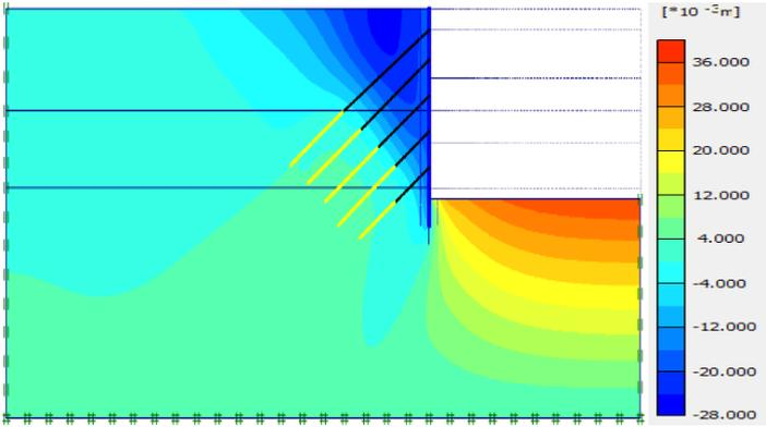
Figure 9 – Vertical displacements in the last phase (max= 28mm)
