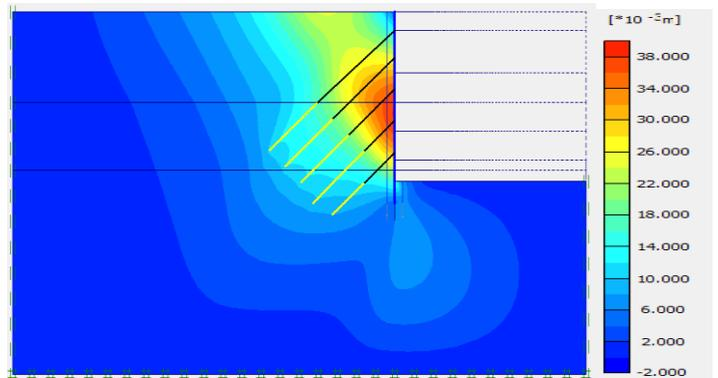
Figure 8 – Horizontal displacements in the last phase (max= 40,14 mm)
