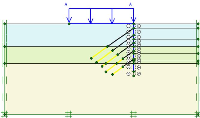
Figure 7 – Geometry of the model simulated in the FEM program Plaxis 2D
