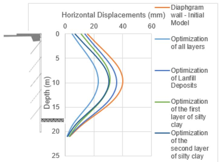
Figure 10 – Horizontal displacements in depth for the model before and after the back analysis
