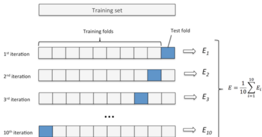
Figure 15: 10-fold cross-validation, used to calibrate our model parameters and to choose the optimal feature set [25].
