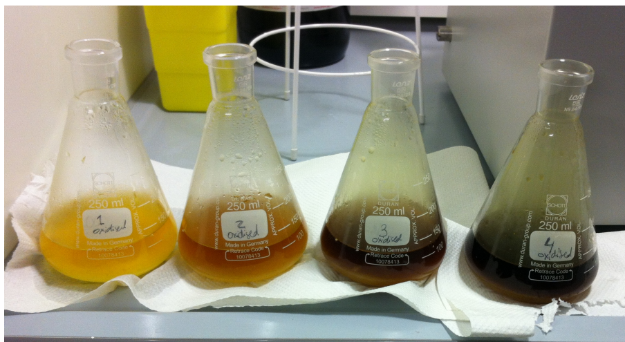
Figure 4.1: Samples 1 to 4 (left to right) of the oxidised cellulose beads. The \text{NaClO}_2 increases from left (i.e. sample 1) to right (i.e sample 4) of the oxidised cellulose beads.
