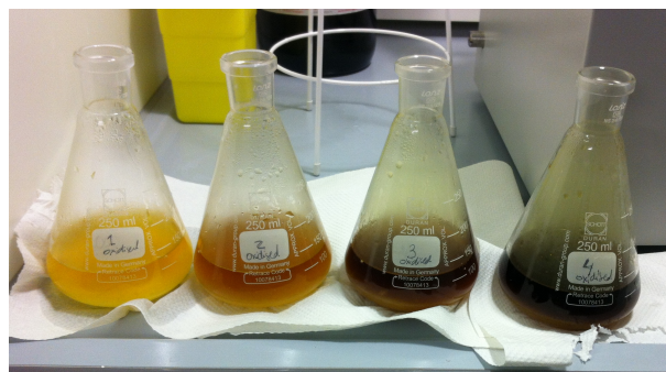
Figure 3: Samples 1 to 4. \text{NaClO}_2 increases from left (i.e. sample 1) to right (i.e. sample 4) of the oxidised cellulose beads.
