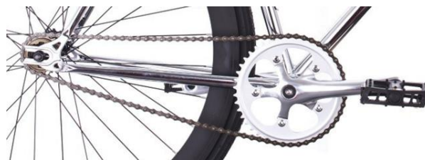
Figure 2.14: Fixed gear system
