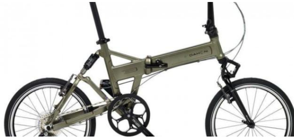
Figure 2.11: Example of vertical folding bicycle.
