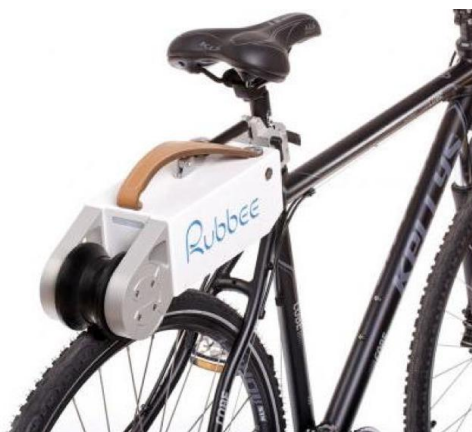
Figure 2.6: Friction drive motor mounted on seat-post. (source: http://electricbikereport.com/electric-bike-motor-comparison/ )
