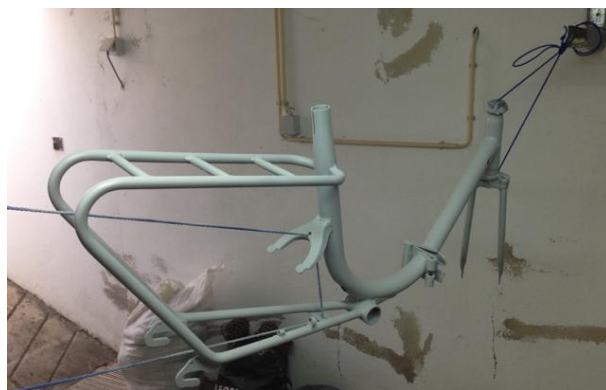
Figure A.8: Primer coat applied to the frame.
