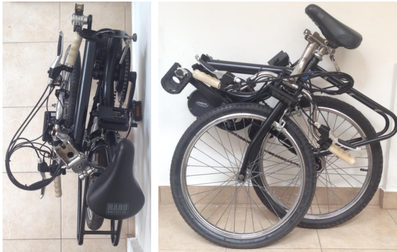
Figure 5.3: Prototype in the folding position
