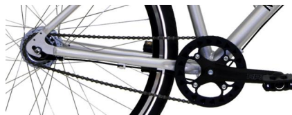
Figure 2.16: Internal gear system
