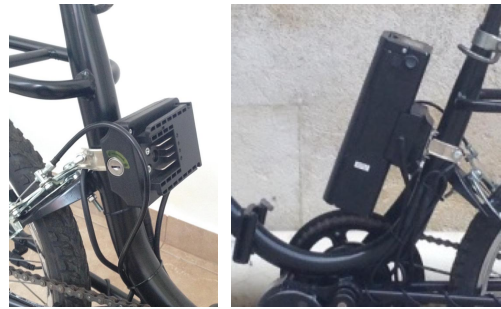
(a) Holder that secures the battery (b) Battery
