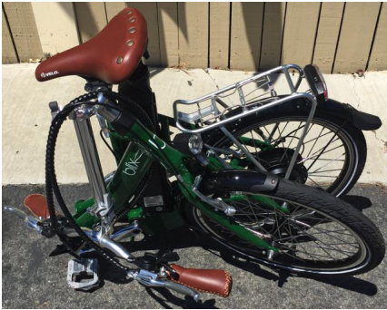
Figure 2.10: Example of horizontal folding bicycle with unaligned wheels.
