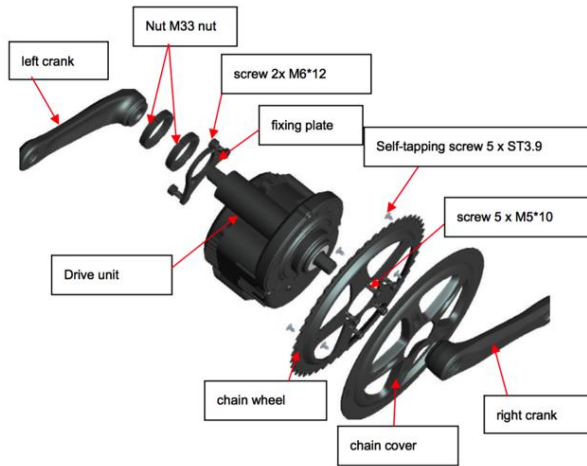
Figure A.3: Exploded view of the motor.
