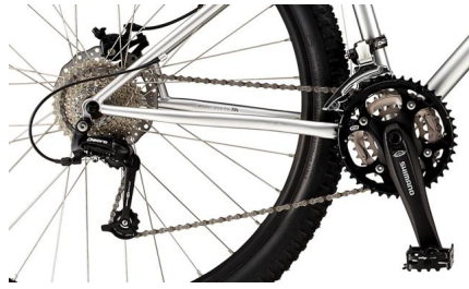
Figure 2.15: Multi-speed gear system
