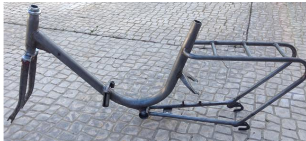
Figure A.7: Frame cleaned and ready for the paint job.
