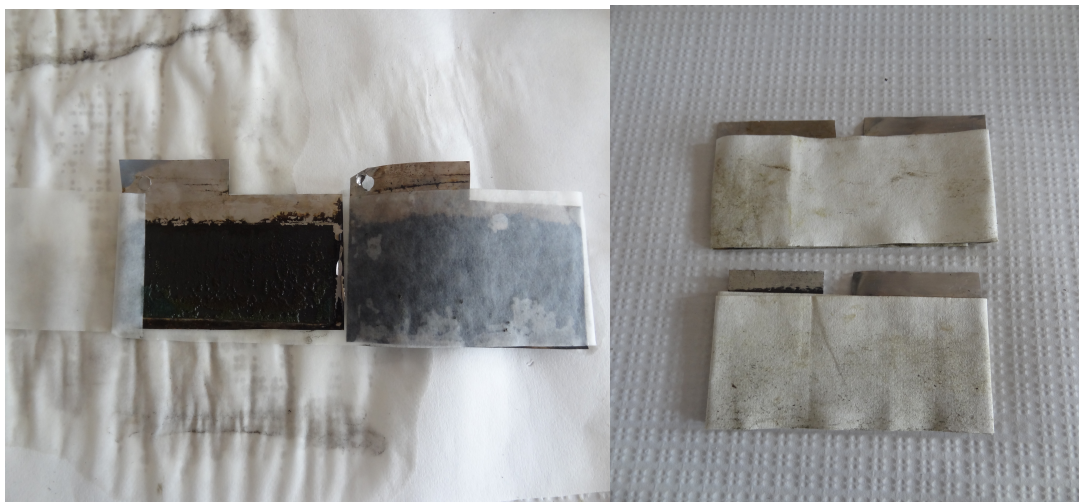
Fig. 28 Assembly of NiCo-NiCo plates (left) and already assembled NiCo-NiCo and NiCo-C plates.
