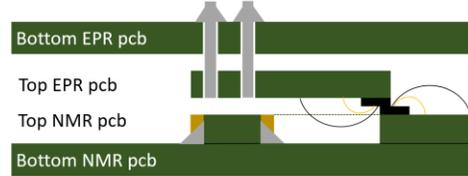
Fig 6- Schematic of the assembly of the PCB's when aligned. Bottom PCB's are 10x1  $\text{cm}^2$  and top ones are 2x1 (EPR) and 3x1 (NMR)  $\text{cm}^2$ .
