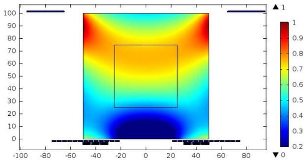
Fig 2- Normalized contribution to the total signal as deduced from  $B_{iLEPR}^2 B_{iLNMR}$ , with the above considerations. Cross section shows the two coils and the  $100 \times 100 \mu\text{m}^2$  capillary used. Dimensions in  $\mu\text{m}$ .
