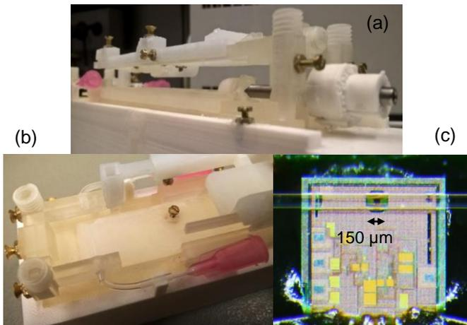
Fig 5- Final prototype seen from the back (a) and the front (b). M1.6 screws used to control friction and to lock movement are shown as well as the adjustment system and capillary interface. Image of the precision achieved when aligning the capillary with the NMR coil (c)
