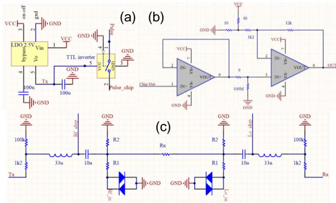
Fig 8- Schematic of the NMR PCB's power management (a), output stage (b) and excitation/downconversion RF input stage (c).
