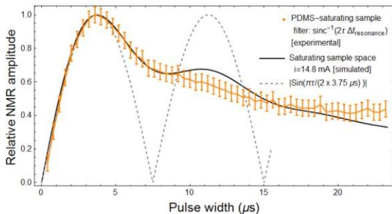
Fig 9- Comparison of experimental, simulated and theoretical, for a single spin, NMR amplitudes with respect to the time of the RF pulse.
