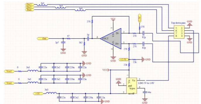
Fig 7- Schematic of the EPR PCB up to the top/bottom pins.
