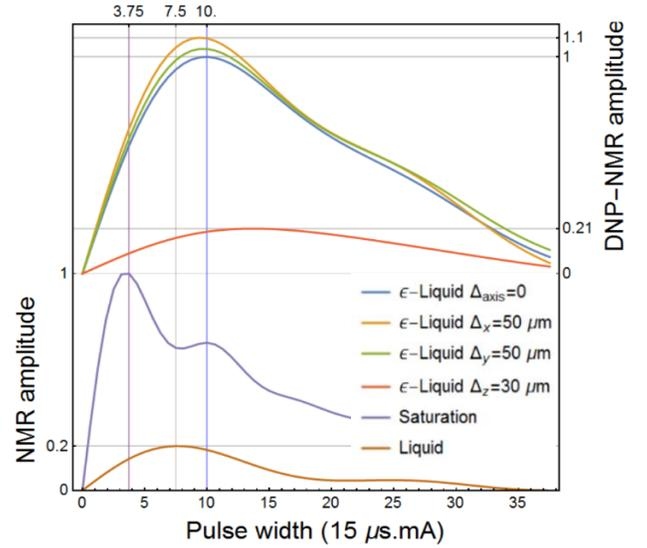
Fig 3- Relative amplitudes of NMR and DNP-NMR signals for different samples, in different spaces, with respect to RF pulse length. DNP-NMR comparison made normalized to axial alignment and capillary contact.
