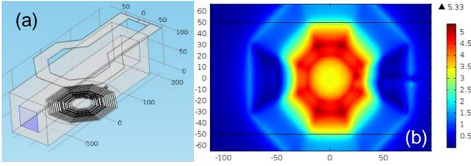
Fig 1- Geometry simulated in Solidworks and imported into COMSOL (a) and transversal unitary magnetic field in the xy plane on the bottom of the capillary (b). Dimensions in  $\mu\text{m}$  and magnetic field in Gauss.
