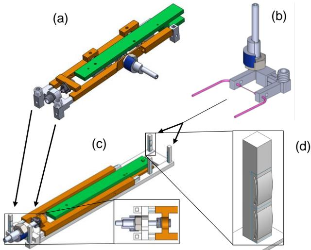
Fig 4- Solidworks model of the system. Table system for the EPR (a) and NMR (c) PCB's (in green), the microfluidic system (c) and detail of its attachment (d). Arrows indicate the correct placement of each part.
