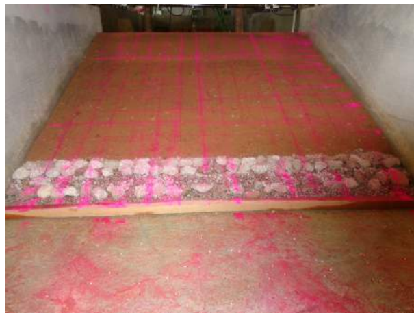
Figure 3.19: Drain placed at the toe of the embankment model.
