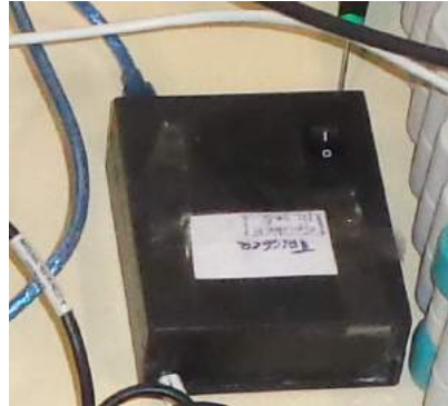
Figure 3.6: Analog Trigger for data synchronization
