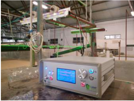
Figure 3.10: Laser used for dam breach monitoring
