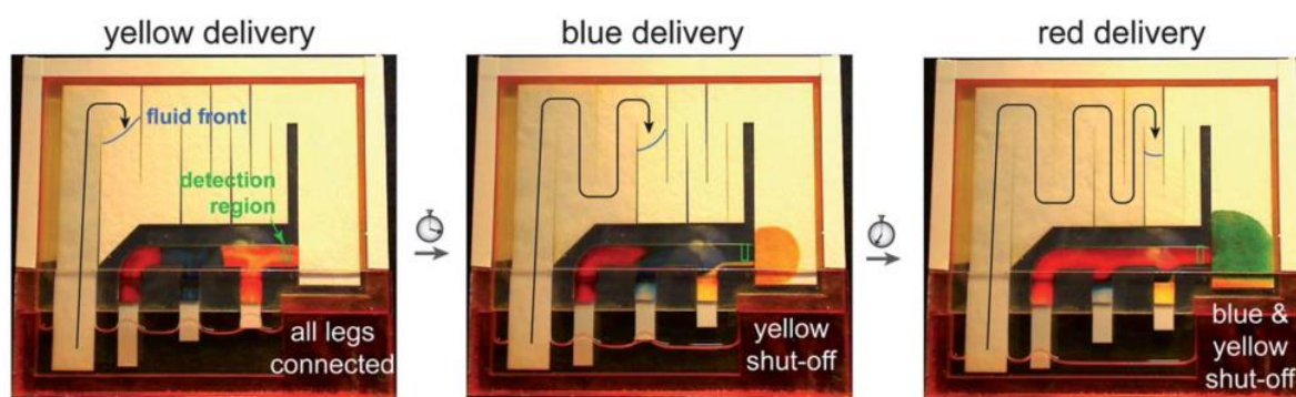
Figure 1-6 Autonomous fluid delivery in a 2DPN. Each leg wicked fluid from a single buffer source, and dried dyes representing reagents create different fluids from each leg (colours). Each coloured fluid arrived at a different time at the “detection zone” (green box) and was shut off in a timed sequence after delivery. Adapted from [22]
