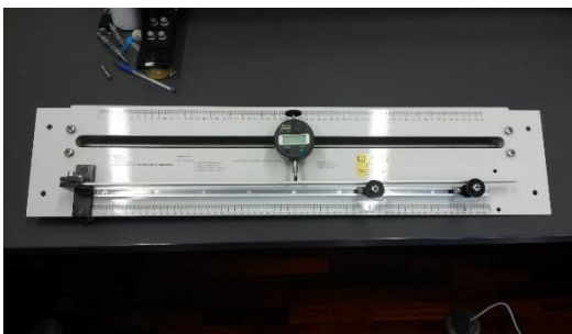
Figure 12 – Deflection of beams
