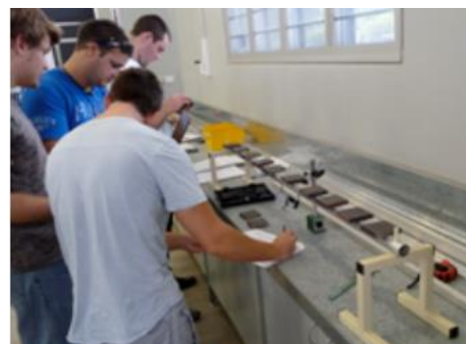
Figure 22 – Deflection in beams
