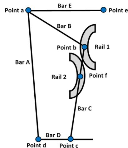
Figure 1: Draft of the device with key points, bars and rails
