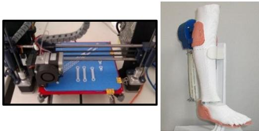
Figure 6: 3D printing – parts of the orthosis; functional prototype
