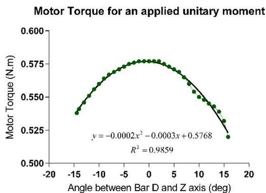
Figure 4: Relation between motor torque and rotation angle of bar D for a unitary moment
