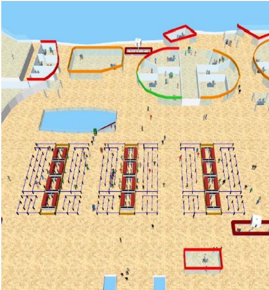
Figure 9. Landside of the departure terminal, as seen on AnyLogic software - 3D animation (Cheng, 2014)
