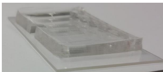
Figure 1.17 Example of a PDMS-glass microfluidic device
