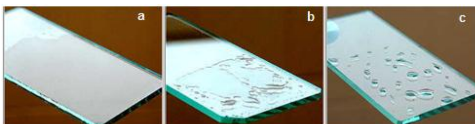
Figure 1.16. Spreading effect of a water droplet in glasses cleaned with a combination of cleaning method and UV/Ozone (a), only wet cleaning (b) and unprocessed (c), respectively [40]
