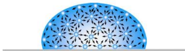
Figure 1.4. Representation of unbalanced forces that create surface tension [21]
