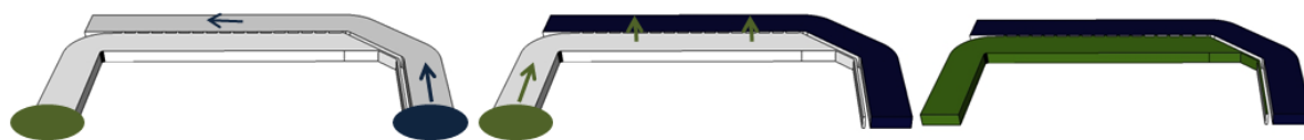
Figure 2.19 Illustration of the fluid flow through the 1 st and 2 nd inlets of the sequential module
