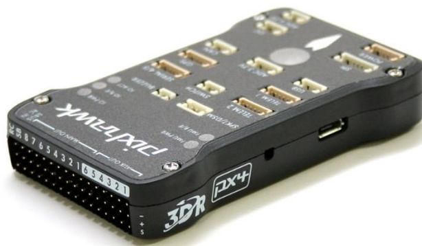
Figure 11 - The Pixhawk autopilot board
