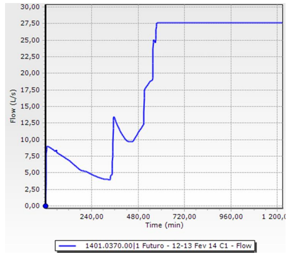
FIGURE 11 – Operation of vortex valve installed in Emissário 1 weir.
