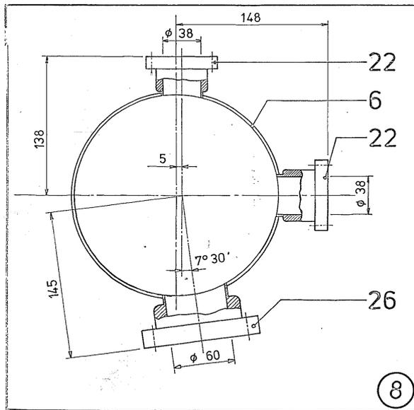
Figure 1: Tokamak ISTTOK's port 8, where the pin-hole cameras are installed. Note the LFS deviation of the bottom view.
