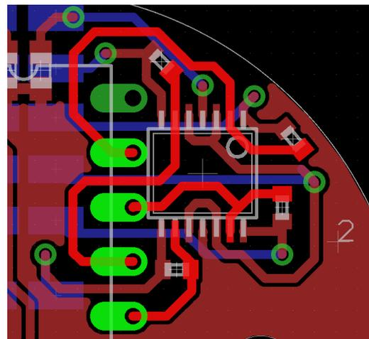
Figure 4: Detail of the PCB board, highlighting the tracks whose length was minimized. At the center, a OPA4354 SMD integrated circuit is visible, surrounded by four 0402 resistors.
