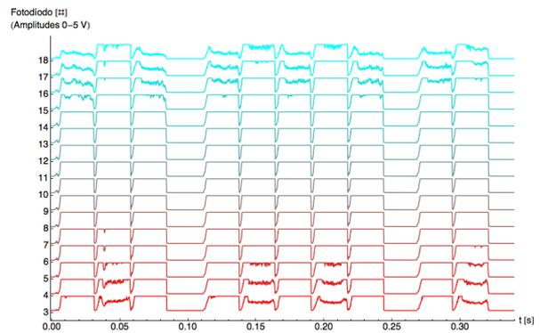
Figure 8: Example results for shot #38234 (equatorial view) showing overall signal saturation.
