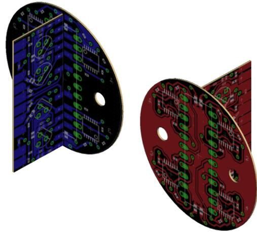
Figure 3: The resulting PCB board, back (left) and front (right). The two holes are for the two M4 screws fixture. These boards are kept in the vacuum vessel.
