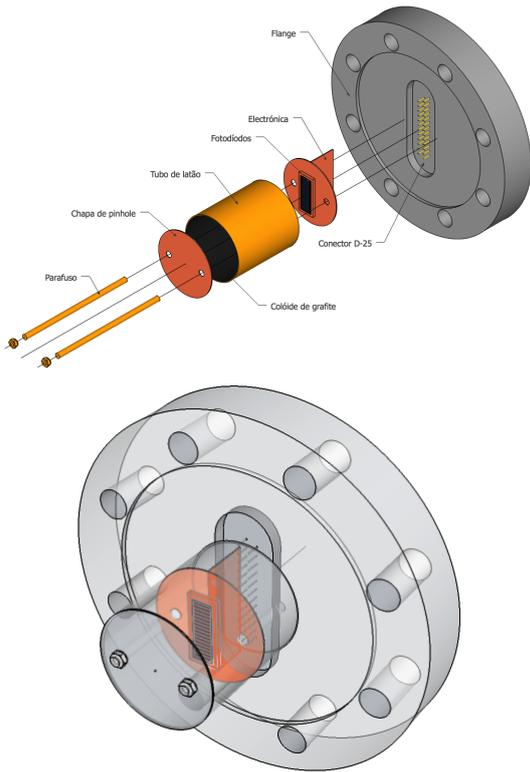
Figure 5: How it all fits together. Top: Exploded view of the tomographic cameras, showing from right to left: vacuum flange with DB-25 data feedthrough, PCB with photodiode array, brass tube with graphite colloid, pinhole and supporting screws and nuts. Bottom: compact transparent display of the camera.
