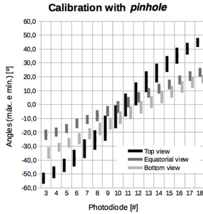
Figure 7: Results for the pinhole calibration, in which the role of the graphite colloid is visible in those cameras that have this finishing (equatorial and bottom views).
