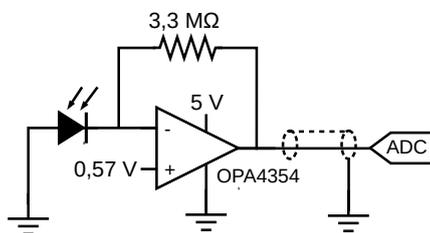
Figure 2: The implemented transimpedance amplifier circuit.
