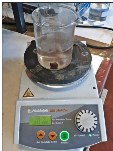
Figure 17. Salt removing process carried out with magnetic stirrer.
