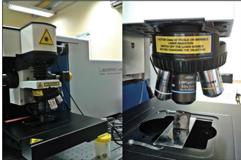
Figure 20. LabRam HR Evolution Raman Spectrometer (left); objective 50X focused on the sample (right).
