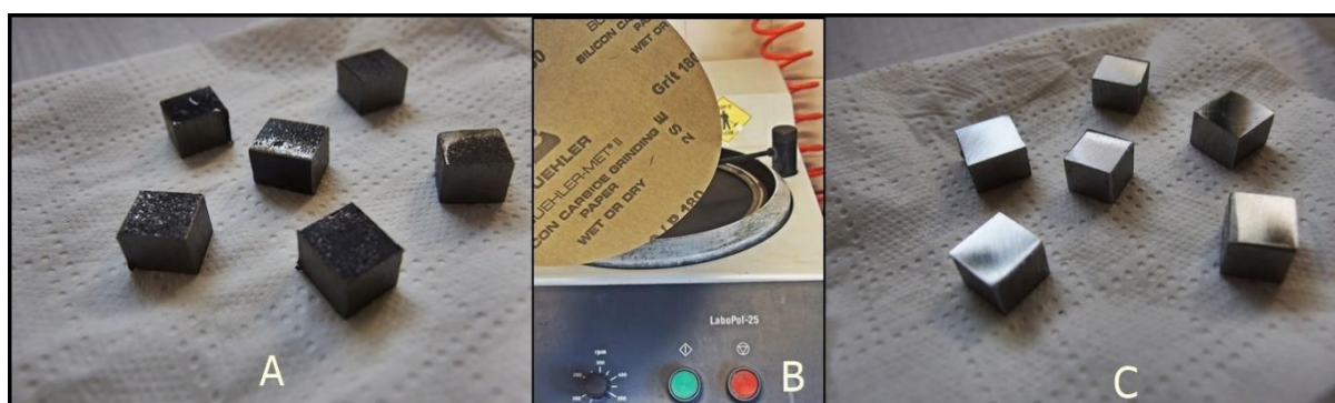
Figure 13. A – Steel specimens in as-received condition after cutting; B – Polishing paper and LaboPol-25 machine; C – polished steel specimens.
