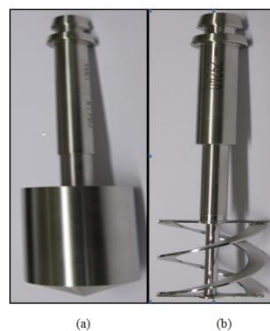
Figure 4.3: a) Cylindrical spindle CC27-SN27965, Fa. Anton Paar, b) Double helix spindle ST24-2HR-37/120 SN29240, Fa. Anton Paar
