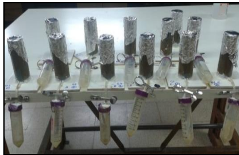
Figure 7 - Samples prepared for the MICP treatment (Phase IV)
