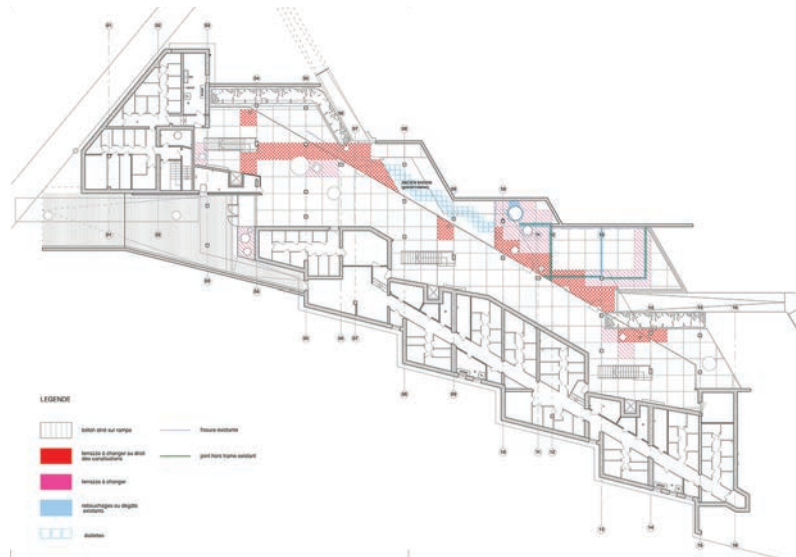
157. Detailed construction drawing of the works on the flooring of the Miremont's hall 1:800. (Meier+associés architectes, August 26 th 2013, original scale 1:200). Grey: striated concrete over the ramp; Red: terrazzo to replace due to the works on the piping system; Pink: terrazzo to replace; Blue: cracks to refill; White with blue line: new passage to be built over the water basin; Blue line: existing cracks.
