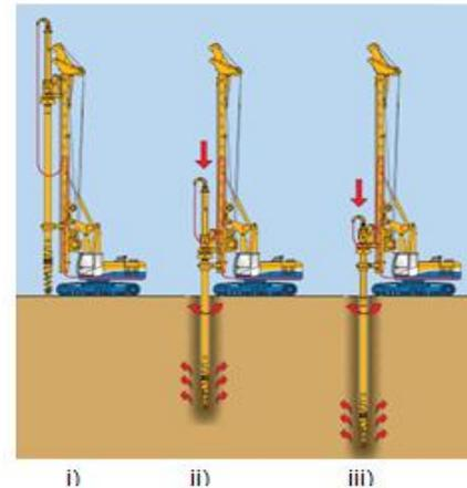
Figure 2 - Initial stages of the FDP installation process.
