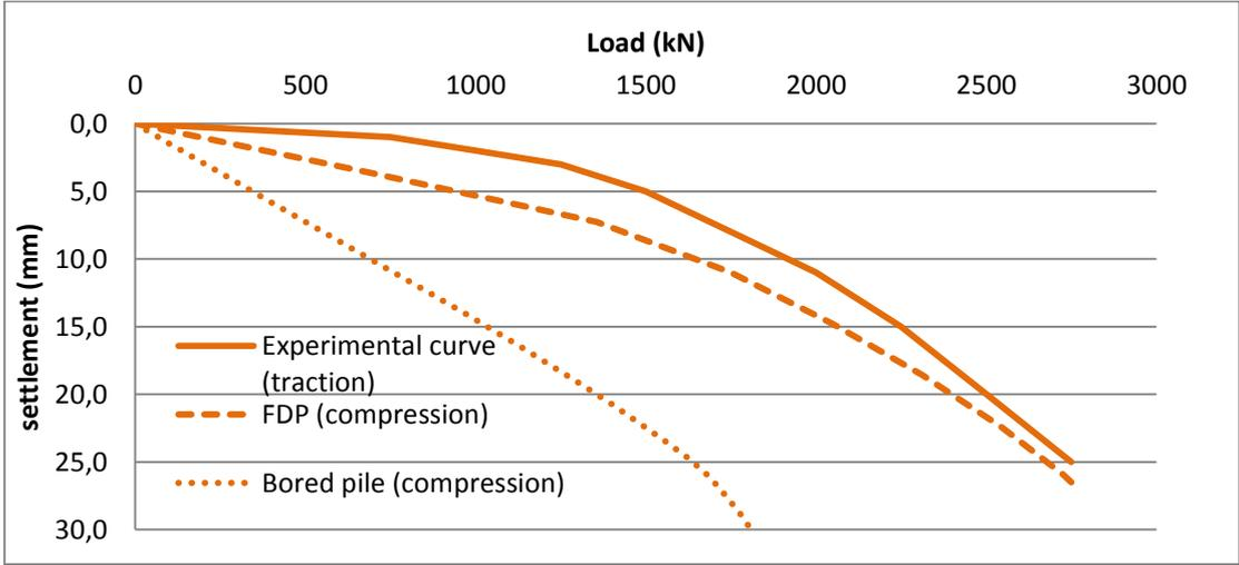
Figure 7 - Load-settlement curves of the numerical and experimental solutions
