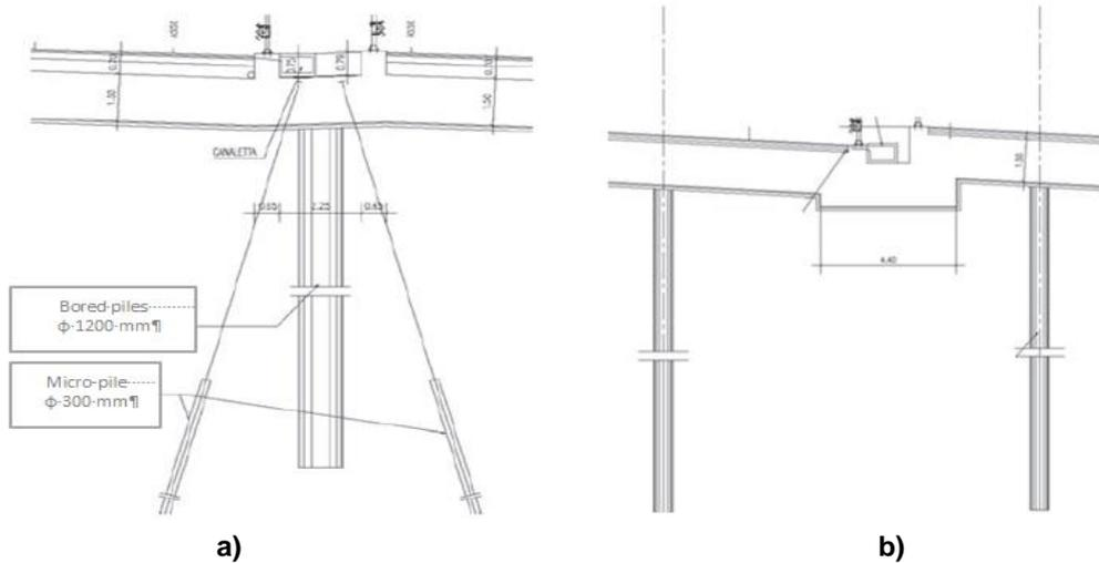
Figure 4 - Installation detail - a) of bored piles and micropile solution; b) with FDP (Bringiotti et al, 2008)
