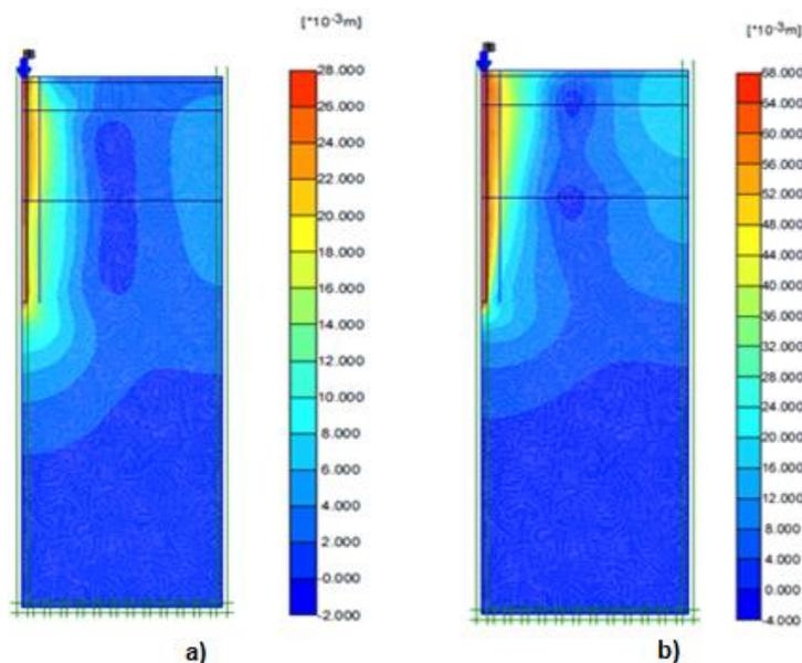
Figure 6 - Total displacement during the static load test a) FDP model; b) bored pile model
