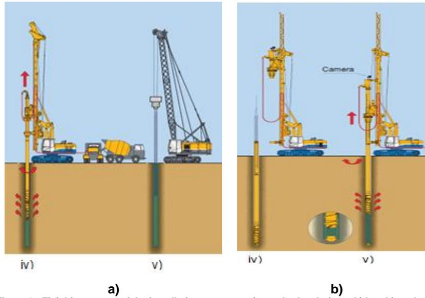
Figure 3 - Finishing stages of the installation process - a) standard technique; b) lost bit technique
