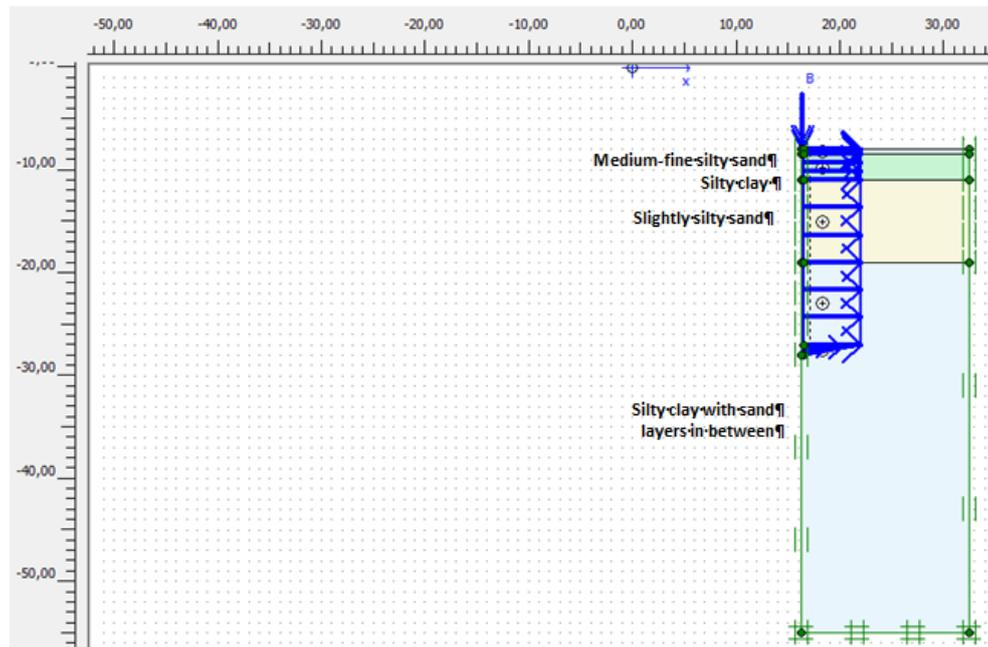
Figure 5 - Representation of the numerical modelling of an FDP (*Plaxis 2D software*)
