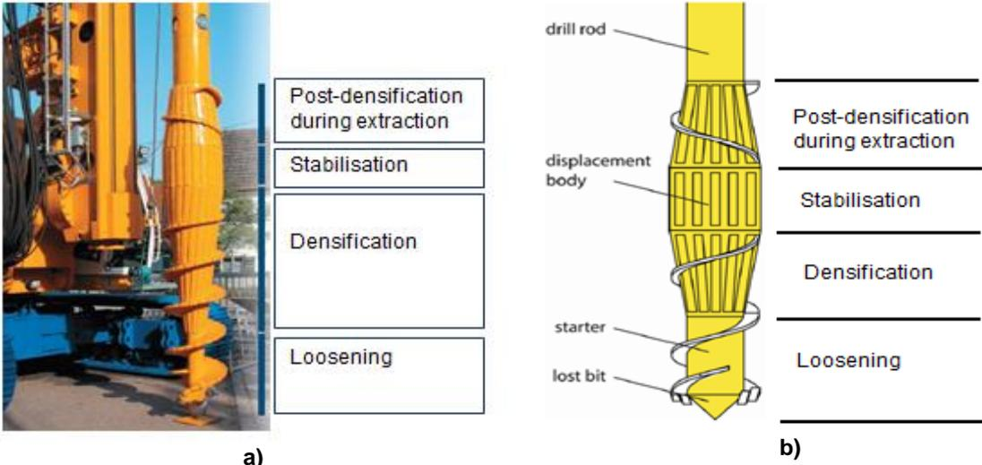
Figure 1 - Implements and respective functions which constitute the drilling tool - a) standard technique (Bauer Maschinen GmbH, 2013); b) lost bit technique (Busch, 2009)
