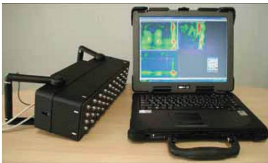
Figure 3.6 - Antenna and laptop with control and analysis program. [Catalog NDT, 2010]
