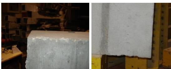
Figure 4.3 - Peeling and delamination in the prototypes
