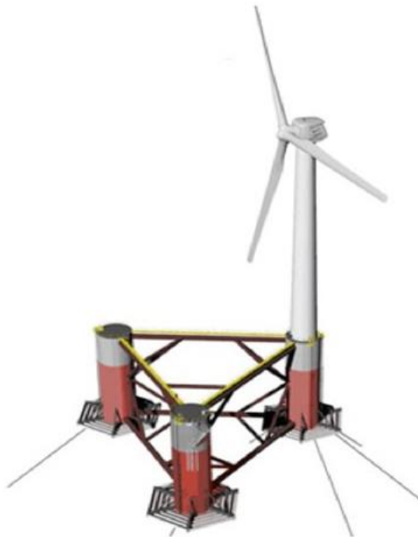
Figure 1-4 The WindFloat platform (Bornemann, 2011)
