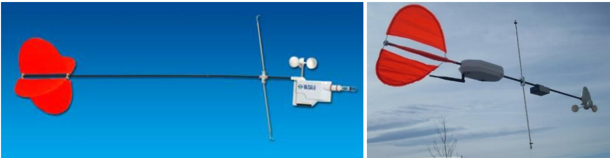
Figure 14: Tethersondes by Vaisala (left) and Anasphere (right)
