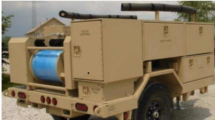
Figure 17: Heavy duty aerostat launcher from Skydoc (Steffen 2014)
