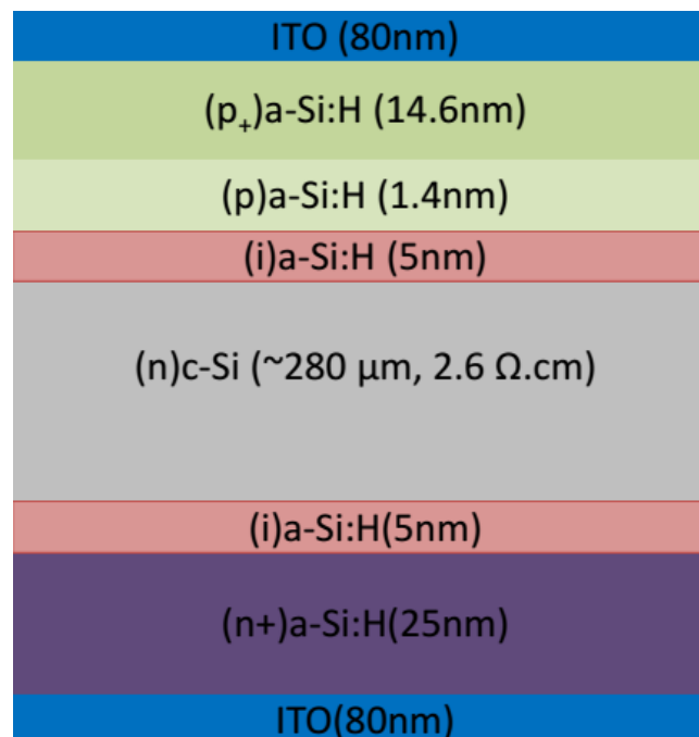
Figure 3.10 Structure of optimized standard cell precursor showing the dopant gradient
