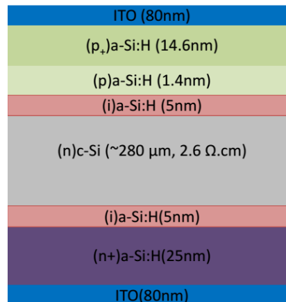
Figure 8 Structure of optimized standard cell precursor showing the dopant gradient
