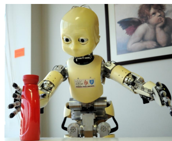
Fig. 1: The iCub humanoid robot performing a reaching task.
