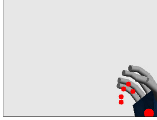
Figure 5.1: Estimated positions of the fingers tips (in red dots) at filter initialization. Note the difference to the real pose show in the simulator.
