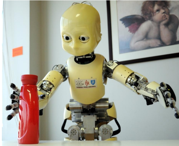
Figure 1.1: The iCub humanoid robot performing a reaching task.
