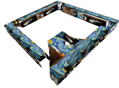
Figure 10: Overview of corridor 3D model, built from the first 112 "synthetic" images with Kinect equivalent error added.
