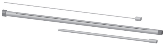
Figure 2. 3D visualization of the ribbon burner (center) and of the materials for structural interventions in the oven (top: gas limiter; bottom: gas guider).
